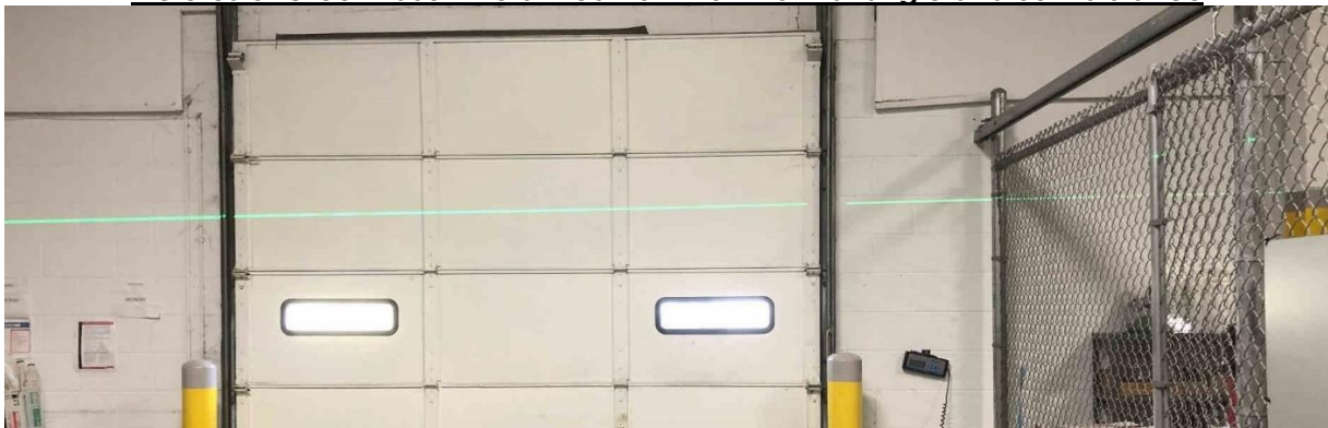
Pictures of Green Laser line aimed from non-normal angle and 50 ft distance
